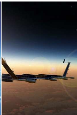
SolarEagle (Boeing/DARPA) WSP: 120m Weight: 900kg
