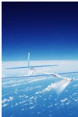
Solara 50 (Google/Titan Aerospace) WSP: 50m Weight: 90kg
