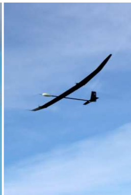
PHASA-35 (BAE Systems) WSP: 35m Weight: 149kg
