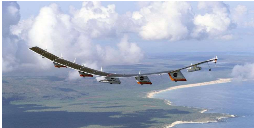
Helios, (NASA/AeroVironment) WSP: 75.3m Weight: 600kg
