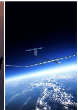
Zephyr-S (Airbus) WSP: 24m Weight: 72kg
